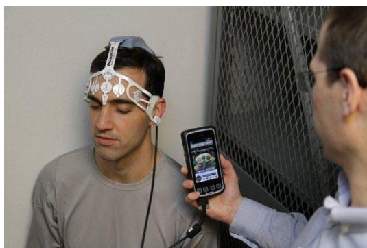
The Ahead 200 uses commercial smartphone technology to analyze a patient's brain activity for signs of a traumatic brain injury within 24 hours of the injury.
